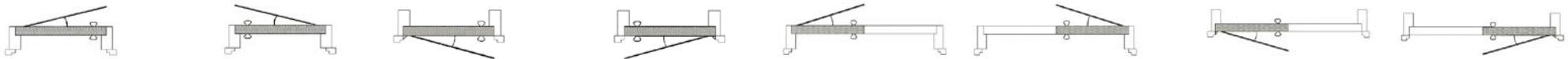
LEFT-HAND INSWING RIGHT-HAND INSWING RIGHT-HAND OUTSWING LEFT-HAND OUTSWING LEFT-HAND INSWING RIGHT-HAND INSWING RIGHT-HAND OUTSWING LEFT-HAND OUTSWING
