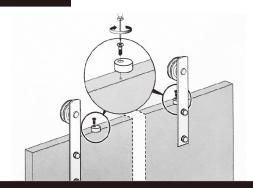
Position and secure each anti-jump block at least I" from the edge of the straps.
