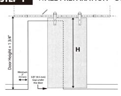
Position the rail by measuring up from the door height (H) + 1-3/4" to the center of the rail. Ensure there is a gap of 3/8" at the bottom. Lastly, ensure the rail is level and leave a minimum of 2 1/4" from the end of the rail to the side of the opening (as shown). If installing with an opening for 80" standard door size, remove the top trim and cut the side trim horizontally along the height of the opening.
