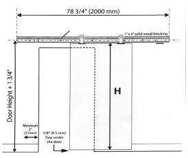
A. A solid wood Mounting Board is required to be mounted to the drywall before proceeding with the rail installation. Position the Mounting Board by measuring up from the door height (H) + I-3/4" to the center of the rail/Mounting Board. Ensure there is a gap of 3/8" at the bottom. Lastly, ensure the Mounting Board is level and leave a minimum of 2" from the end of the Mounting Board to the side of the opening (as shown).
