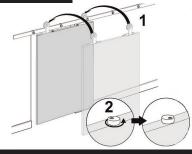
Position the assembled door onto the secured rail and tighten each anti-jump block. Ensure all parts are operating correctly by sliding the door side to side.
