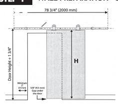
Position the rail by measuring up from the door height (H) + 1-3/4" to the center of the rail.
