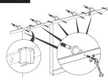
Install rail centered onto the Mounting Board, using the provided lag bolts and anchors if needed. Align each lag bolt and spacer to the rail holes, secure with a wrench. (Note: Wide end of round spacer goes toward wall)
