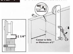
HORSESHOE & DIAMOND DESIGN INSTRUCTIONS: Determine roller location in field, on a per door basis. Position the roller at least I-I/4" from door edge. Mark holes with a pencil and predrill holes, then secure into place.
