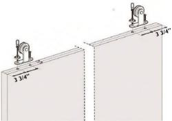
Position each roller a minimum of 3 3/4" from the edge of the door.
