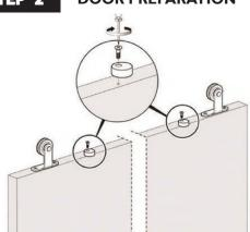
Position and secure each anti-jump block at least I" from the edge of the straps.
