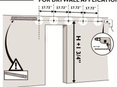
Center the rail on the Mounting Board as directed in Step 3. (Door Height +1-3/4") Ensuring levelness, mark the holes using a pencil and pre-drill holes into the Mounting Board.
