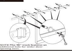
Install rail centered onto the Mounting Board, using the provided lag bolts and anchors if needed.
