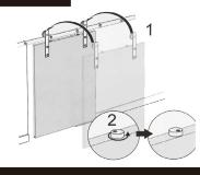
Position the assembled door onto the secured rail and tighten each anti-jump block. Ensure all parts are operating correctly by sliding the door side to side.
